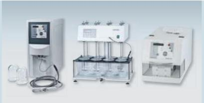
allows the baskets/paddles to be pushed upwards to gain maximum accessibility to the vessels.
